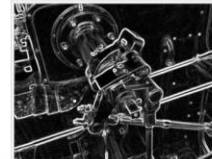
The Sobel operator applied to a colour photograph of a steam engine. (See the original image here .)
